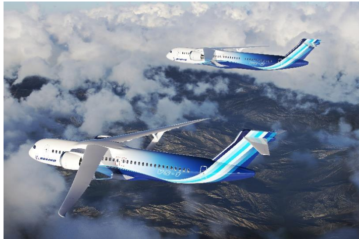
Artist concept of commercial aircraft families with a Transonic Truss-Braced Wing configuration from the Sustainable Flight Demonstrator (SFD) project. The new project was announced in January. Credits: Boeing
